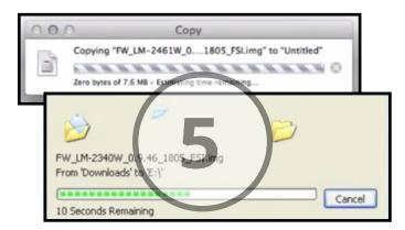
Copy / Paste or Drag and Drop the unzipped .img Firmware file to the monitor.
