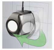
If using an i1D3 OEM please make sure to open the diffuser covering the probe's lens before starting calibration. The lens should be pointing towards the screen and the white diffuser disk should be pointing away from the screen.
