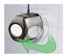
If using an i1D3DS OEM please make sure to open the diffuser covering the probe's lens before starting calibration.
